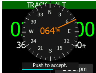
Figure 2: Direction rose is shown for more intuitive target track selection. The orange line points to the new target track selection and its numerical value is shown in the middle.
