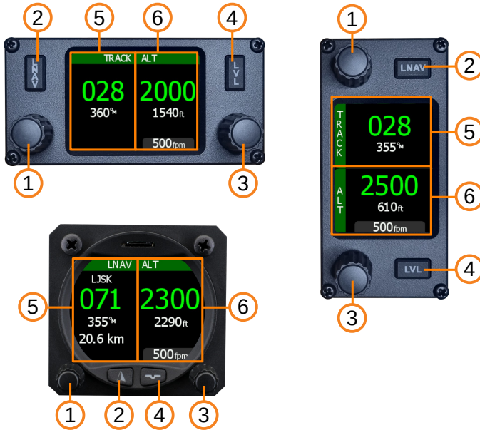
Figure 1: Amigo controls and screen layout organization. Vertical Amigo has layout split vertically: track and LNAV on top and altitude on the bottom. Other Amigos (horizontal and round 57 and 80) have layout split horizontally: track and LNAV on the left, altitude on the right.
