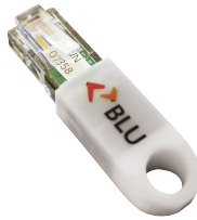
Figure 19: A small CAN bus to Bluetooth bidirectional interface module.
