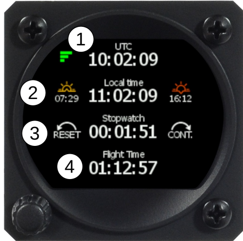
Figure 27: Horis chrono screen with markings.
